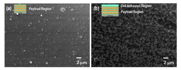
**Fig. 2** SEM images of **a** substrate/(PDAC/PSS)<sub>10.5</sub>(PMAA/PAAm/PMAA/PEO-*b*-PCL<sup>dex</sup>)<sub>20</sub>(PMAA/PAAm)<sub>3.5</sub> and **b** substrate/(PDAC/PSS)<sub>10.5</sub>(PMAA/PAAm/PMAA/PEO-*b*-PCL<sup>dex</sup>)<sub>20</sub>(PMAA/PAAm)<sub>3.5</sub>(collagen I/HA)<sub>4.5</sub>. Both images are measured as prepared
